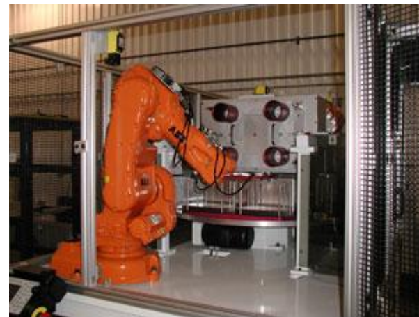
Robotic tending of an injection molding machine, courtesy ABB Inc.
